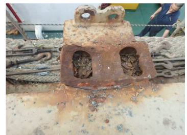
Clear evidence of the forced removal of a 'locked' twist lock
