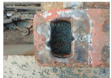
Clear evidence of the forced removal of a 'locked' twist lock
